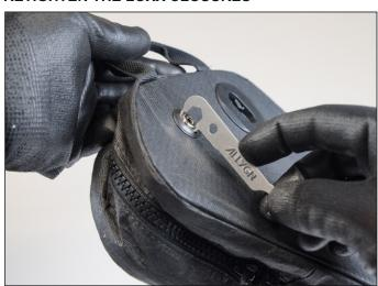
In case the Loxx fasteners on the Micro Panniers come loose or need position adjustment, you can use the two pins on the Micro Tool to tighten the outer lock ring. The Loxx fastener's position can be adjusted 1mm in all directions for best fit.
