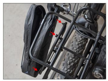
There is matching left and right Micro Pannier for each Micro Rack. Simply place the corresponding Micro Pannier on the two magnetic Fidlock Snap bolts of the rack, and it will snap into place.
