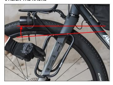
Place your bike on a flat surface and rotate the Micro Racks until the top sides are parallel to the ground. Tighten the bolts to the torque values recommended by your fork's manual, usually between 2Nm and 5 Nm. Check all bolts regularly after riding to make sure they are still tight.
