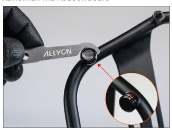
In case the Fidlock Snap bolts come loose, undo the bolt using the Micro Tool by hooking it into the 2mm hole on the side of the Snap bolt. Apply Loctite or similar on the threads and fasten it again with 5Nm.
