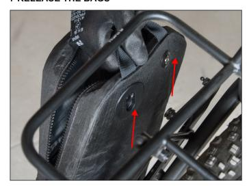
Now pull up on the handle of the Micro Pannier to slide it out of the Fidlock Snap bolts.
