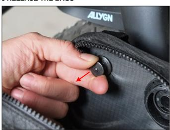
To release the Micro Rider Panniers from the rack, open the bag and pull on the Loxx button to unlock it.
