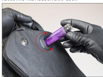
The Fidlock Snap locks on the Micro Panniers may come loose or need angle adjustment to precisely snap to the Micro Rack's Fidlock Snap bolts. To retighten, hold the lockring inside the Micro Pannier with your fingers. You can use a standard lighter to turn or tighten the Snap outer.
