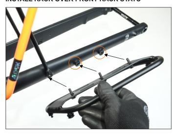
If you are already riding with a Diamond Rack or similar which occupies one of your fork's cargo eyelets, use the included spacers to make up for the thickness of the rack stay and mount the Micro Rider Racks on top of the stay.
