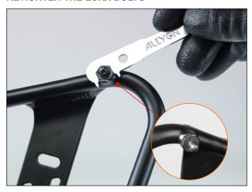
Very rarely, the Loxx bolt may come loose. Use our included Micro Tool (or 9mm wrench) to unscrew it. Apply Loctite or similar on the threads and fasten it again with 5Nm.
