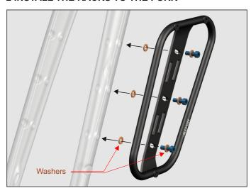
Use the M5 x 16mm bolts with M5 metal washers on both sides of the Micro Rack and bolt it loosely to the fork's cargo eyelets. If your steel fork has only two mounting points you can choose between the upper or lower two holes of the Micro Rack. You must use all three bolts when attaching to carbon forks. Use Loctite 243 or similar on all bolts!
