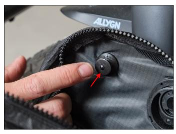
**IMPORTANT!** Before each ride, always ensure that the Micro Panniers are securely snapped in. Actively lock the Micro Panniers by pushing the Loxx button on the inside of the panniers. This is essential for safe riding.
